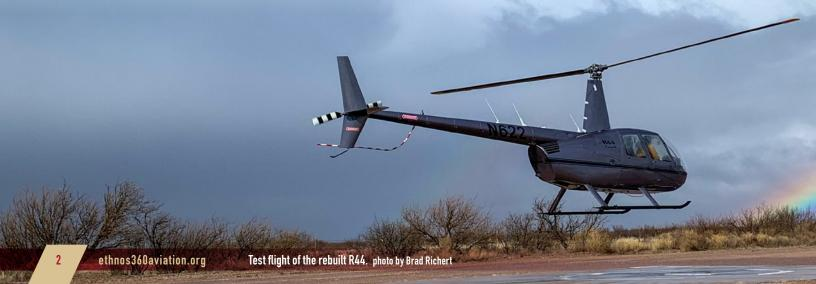
From the skids to the rotors, from wiring to interior, from shaping sheet metal to putting the final touches on the new paint job, our trainees have gotten hands-on experience with every inch of this aircraft. Several of us were holding our breath the other day as the rotors slowly started turning, picked up speed and finally pulled the helicopter upward on its first test flight since the overhaul.
